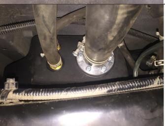
Install the 35mm fill hose onto the tank and the filler neck. Secure using the clamps retained from the removal procedure.
