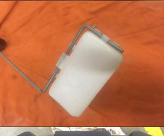
Install the float onto the new float arm as shown.
