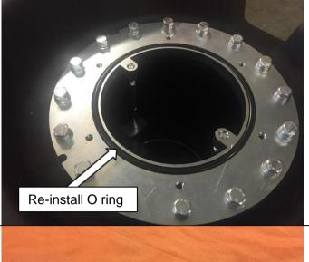
Install the O ring gasket into the groove on top of the Frontier tank.
