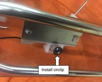
Install the new float arm supplied in the kit to the fuel sender.
