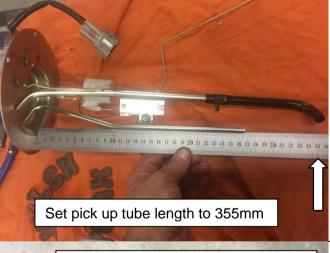
Heat long end of new plastic pick-up tube in hot water. Push the pick-up tube over the end of the steel pick up tube.
