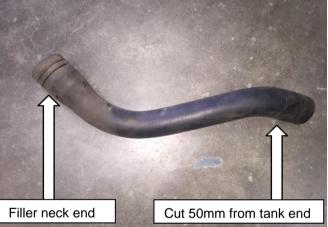
Cut 50mm from the tank end of the 35mm diameter filler hose.
