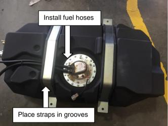
Install the 2 x 450mm long (1/4" and 10mm dia.) pieces of fuel hose onto the fuel sender and secure using the clamps supplied in the kit.
