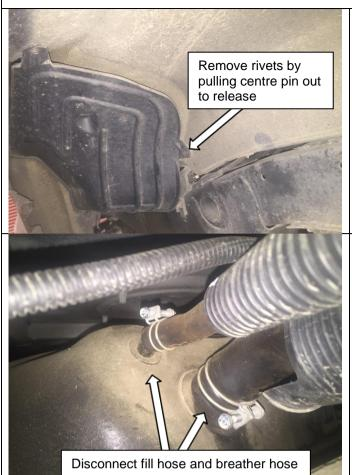
Remove the black plastic trim from the RHR wheel arch by removing the 2 plastic rivets and 1 screw.
