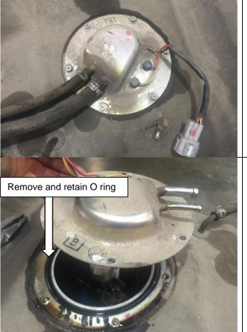
Remove the 6 screws retaining the sender and retain for the installation process.
