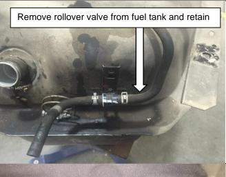
Remove rollover and hose from steel pipe on the fuel tank. Retain hose, rollover valve and clamps for the installation procedure.
