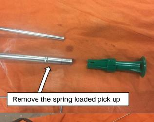
Remove the spring loaded pick up from the steel pick up tube on the sender assembly.
