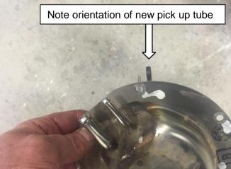
Rotate the pick-up tube to achieve the correct orientation shown in the image
