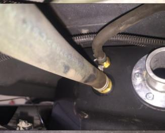
Install the rollover valve hose onto the small brass fitting near the top of the tank, secure using the clamp retained in the removal procedure.
