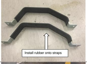
Install the 2 x 800mm long pieces of insulator rubber onto the 2 x top mounting straps as shown.
