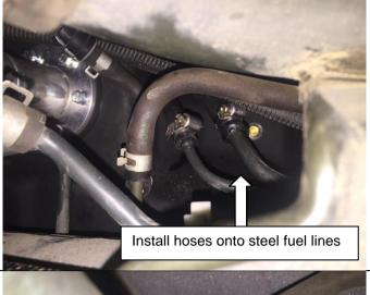
Connect the  $\frac{1}{4}$ " and 10mm fuel hoses from the tank onto the steel pipes on the chassis.
