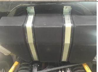
Place the tank onto a jack and raise into position. Place the 2 x lower mounting straps under the tank.
